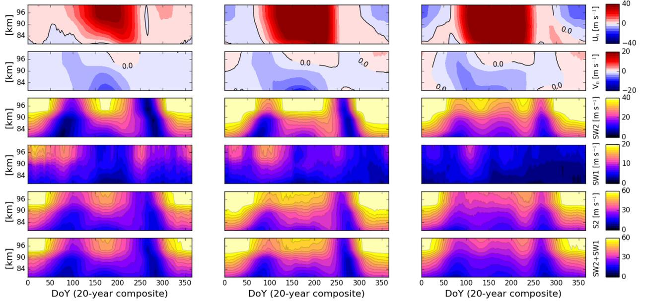
**Figure 3.** HAMMONIA composites of the simulated mean zonal ( $U_0$ ) and meridional winds ( $V_0$ ), migrating semidiurnal (SW2), non-migrating westward propagating wave number 1 semidiurnal (SW1), and total semidiurnal (S2) solar tides, and SW2+SW1, over: (left) Andenes, (middle) Juliusruh and (right) Tavistock.
